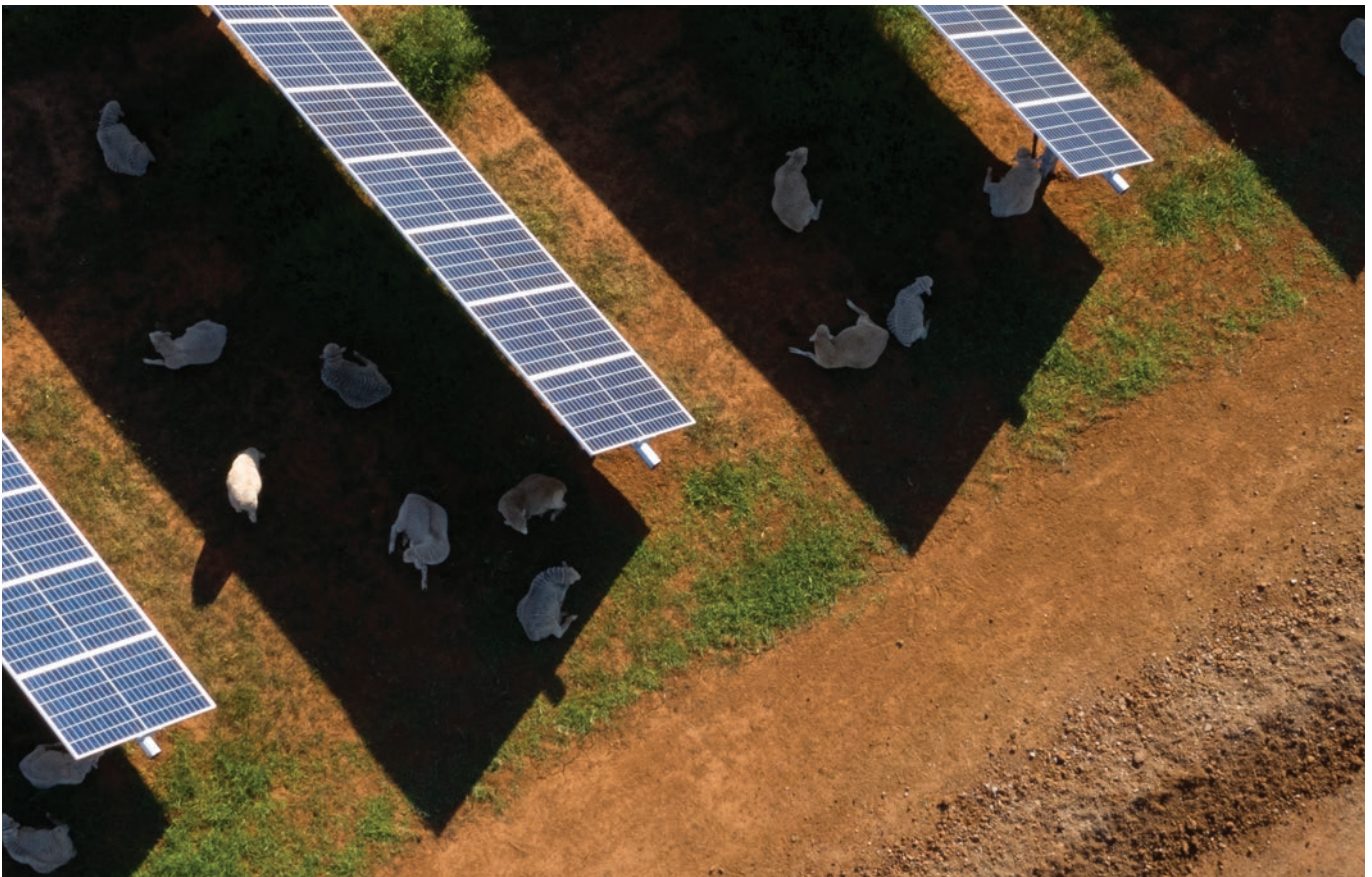
The grazing sheep at Finley Solar Farm in New South Wales are an example of agrivoltaics, which involves a combination of agriculture and solar power production. The panels provide shade for the sheep, and the dual land use means that the farm contributes to both renewable energy and sustainable food production.
